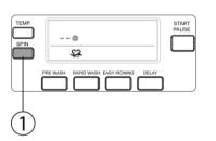
In programmes where the rinse function is applicable, it may be activated by pressing the spin speed setting button one more time after the cancel (--) spin symbol is shown on the electronic display. You know that the soaking function is activated when the symbol Schabes on electronic display.
